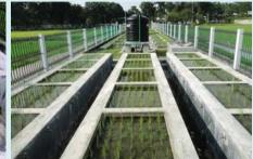
Figure 2: Picture of rice grown in lysimeter for salt tolerant study
